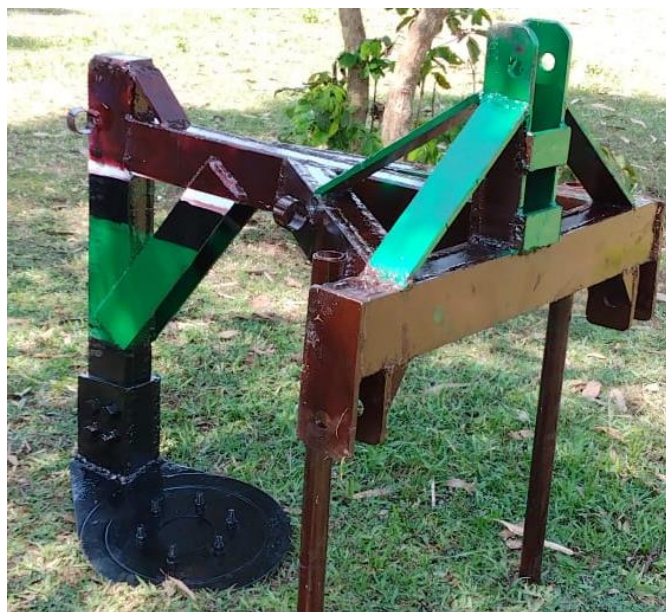
Figure 1. The developed mechanical cassava harvester
